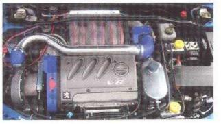
line from tank. Sytec motorsport injection pump, supplying 180 litres/hour at 5 bar. ERL Aquamist race spec water/methanol injection at 2 bar. Highpower Systems 100BHP NOS kit, with Stealth Systems alloy distribution block, progressive controller, direct port injection foggers and combination of stainless steel braided & surgical steel lines with anodised fittings. Alloy distribution block is fitted with fuel & nitrous solenoids at end. either which provides a more and ечеп instant
